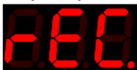
The device will record the modulation output for a duration between 0 to 1000 seconds dependent on the 'Recording Time' set in the menu. The recording can be heard by selecting playback ('P') with the modulation mode switch. The recording will play back continuously and can be trimmed using the trim (sensitivity) control. The recorded waveform cannot be saved. See Understanding recording pg 38
