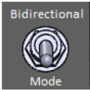
The bidirectional switch is a permanent toggle switch. It is actuated by pushing it backward. It enables modulation output in two directions. Modulating output will normally decrease from 127 to 0 and there will be no further change should the sensor continue below the 0 point. With bi-directional selected, the modulating output will continue to be present in the negative direction. -127 - 0 – 127 . In rotation and guitar-hand mode the bidirectional switch enables a continuous sweep.
