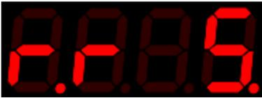
The release rate starts when the sustain time finishes, and sets how long the envelope takes to fall from the sustain level to zero.
