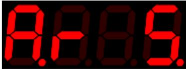
With any modulated parameter, the attack rate sets how quickly the envelope rises from minimum to maximum. It is adjustable from 1 – 99 in 10 millisecond increments with a scale setting of 1, and up to 1 second increments with a scale setting of 99. This provides a total stage time of 99 seconds.
