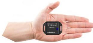
6. Tilt the sensor left, right, forward and backwards and the display will change accordingly.
