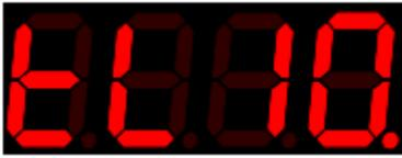
Sets the level at which motion will activate recording. For example, if the record trigger level is set to 10, and recording is armed, recording will start when the current modulation output moves 10 above or 10 below the position recorded when the system was armed. The minimum depth control can also be used to trigger recording.
