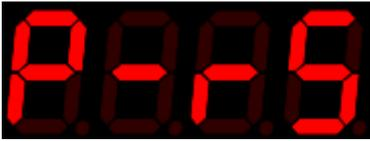
Ring sleeve. The tip is disconnected. This polarity can be used to simulate some footswitches.
