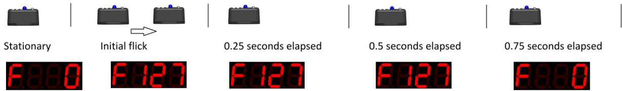
Figure 17 – The ADSR envelope can hold the output at maximum
