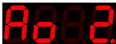
The automatic cut-off parameter determines how long after transmission ceases, the modulating output will reduce to zero. A setting of '0' has no cut-off.
