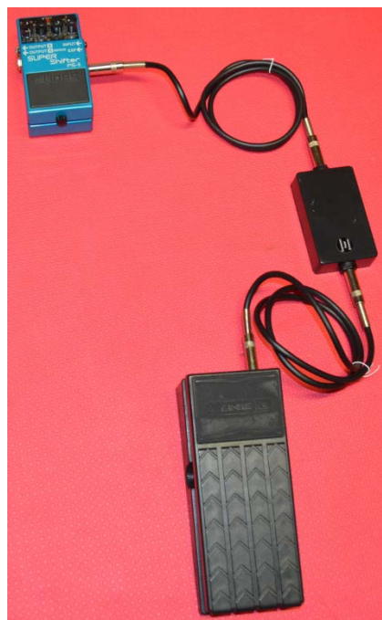
Figure 3 – Insert converter inline between pedal and effect
